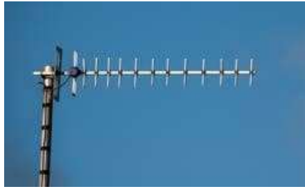
snFig 1: Yagi-Uda antenna showing element types.
